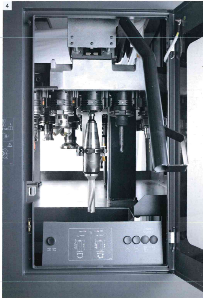
1| Integrated NC rotary table 2| Milling / drilling machining with up to 1,000 rpm 3| Tool magazine with 30 magazine pockets in the standard version, with an optional 60 or 120 pockets 4| Comfortable loading of the tool magazine through a separate door and optional setup aid 5| Integrated milling / turning table
