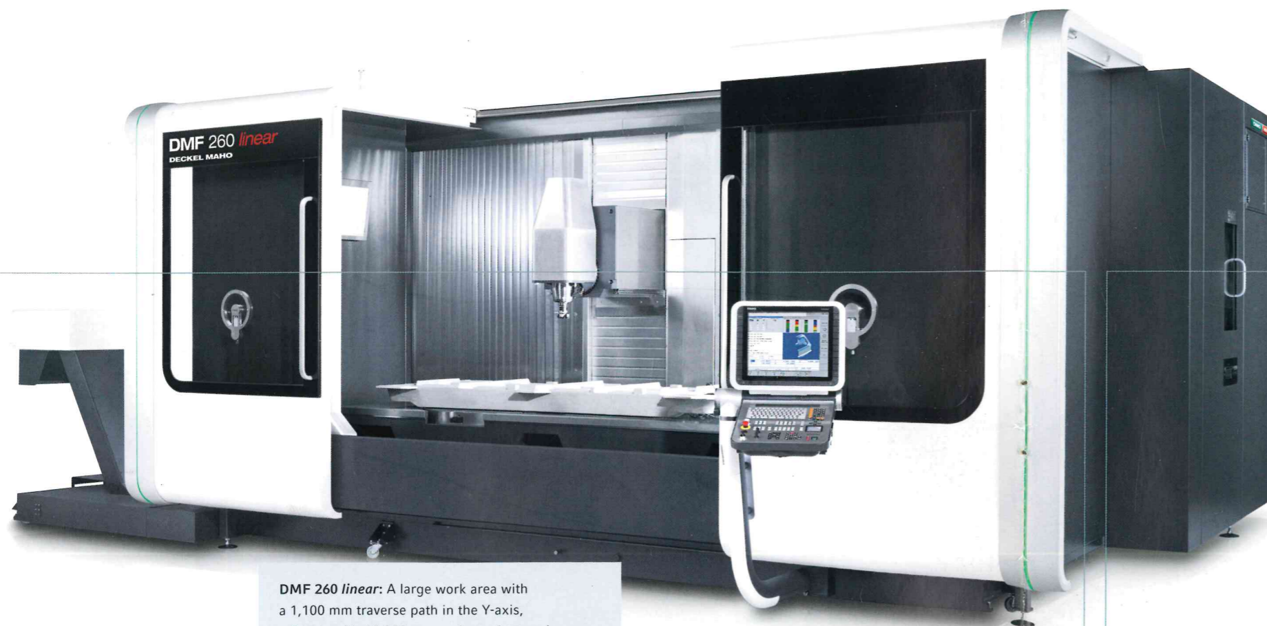
1| Work area with a traverse path in the X-axis up to 3,600 mm, 1,100 mm in Y and 900 mm in Z, for long work pieces and effective twin-table machining with a work area partition wall | 2| Linear drive in the X-axis | 3| Tool magazine with up to 120 pockets | 4| Spindle option: 10,000 rpm motor spindle with SK50 or HSK-A100
