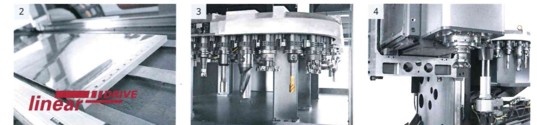
1| Work area with a traverse path in the X-axis up to 3,600 mm, 1,100 mm in Y and 900 mm in Z, for long work pieces and effective twin-table machining with a work area partition wall | 2| Linear drive in the X-axis | 3| Tool magazine with up to 120 pockets | 4| Spindle option: 10,000 rpm motor spindle with SK50 or HSK-A100
