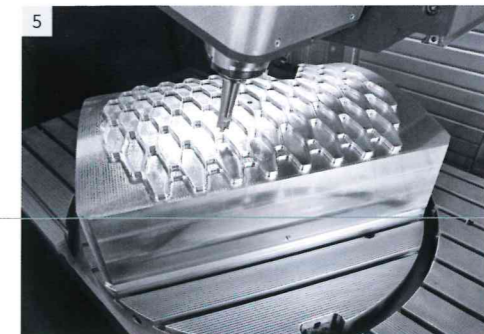
1| Direct measuring systems and linear drive in the X-axis with optional dynamics package 2| Drive in the standard version with a ball bearing spindle 3| Vertical spindle up to 18,000 rpm 4| B-axis 5| Integrated NC-rotary table
